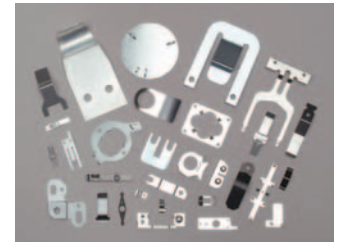
A sample of parts that can be most economically produced by the Fourslide process.
