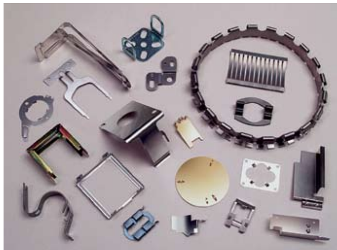
The unique integration of stamping and forming operations makes the fourslide part-making process capable of cutting typical tooling costs to as little as $3,000, halving tooling lead times, and eliminating after-production adjustment to meet specifications.
